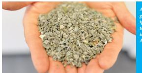
ArcelorMittal uses granulated municipal waste material to substitute coal in its EAF (photo: ArcelorMittal)
