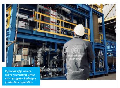
The "scalum" modules from the supplier of world-leading technologies for high-efficiency electrolysis plants can be used to produce green hydrogen on an industrial scale. The company needs the alkaline water
